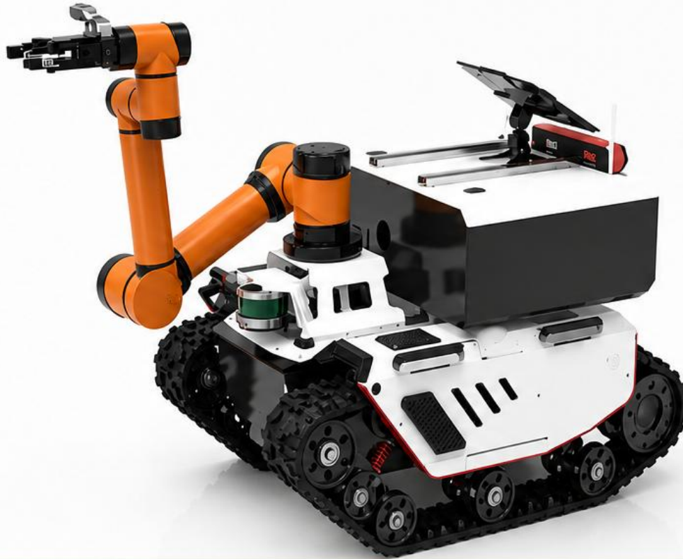
Tracked mobile platform, modular arm — RICS Smart Farm 4.0 .
